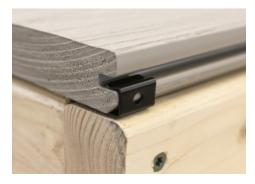
To install, users line up the clip with the back edge of the joist and the center of the cross joist, fasten the clip at the cross joist, and then tilt and insert the deck board into the clip. Each package of Starter Clips contains 25 clips and 25 screws manufactured from 304 stainless steel, enough to cover 30 linear feet. The MSRP per pack is \$19.95. camofasteners.com
